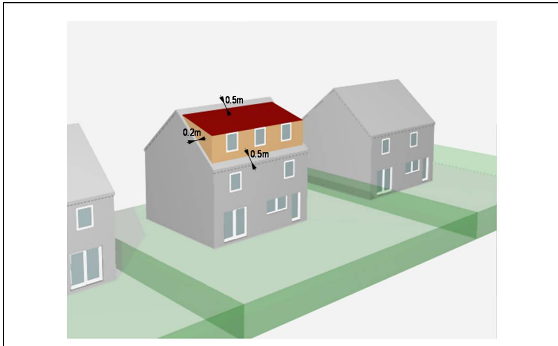
Figure 9: Rear Dormer Extension
